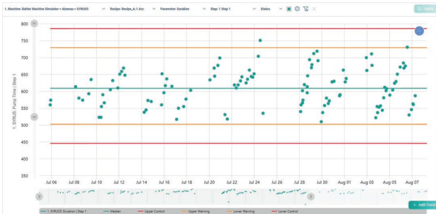
Fig. 2: Exemplary control chart from Bühler Leybold Optics database cockpit. The data shown here simulate the cycles of increasing pump-time from batch to batch till next cleaning run simulated data, as no real customer data can be shared here.
